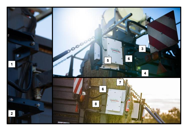
12. Run the flexible conduit that contains the microwave cable over the top of the rear baler frame and connect it into the antennae (#6). You may need an adjustable wrench to tighten the conduit nut inside the antennae. Secure the conduit in place using large cable ties around the baler frame. Connect the microwave cable to the SMA connector inside each antenna, taking care as per the special note about the microwave cable in the Owner's Manual (section 2.2).
