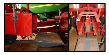
2. Install one side of the bracket kit, with the top two central bolt holes on the top of the bale chamber. Secure with M10 x 25mm Cup Head bolts, flat washer and Nyloc nut.
