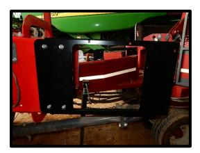
3. Install polycarbonate window and secure with M8 x 25mm bolt, flat washer, spring washer and nut.
