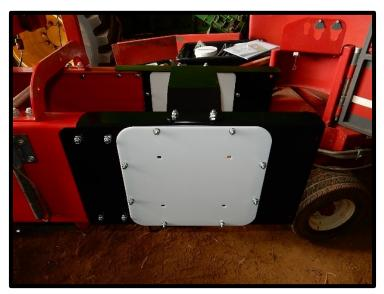
6. Attach the standoffs to both antenna's using MIO x 30mm button socket cap screw, flat washers and spring washers. Then, mount the antennae to the polycarbonate window using the rest of the MIO x 30mm button socket cap screws, flat washers and spring washers. Note: the active antenna (housing with electronics in it) should be on the right-hand side of the baler and the passive on the left-hand side.
