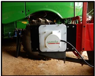
7. Uncoil the microwave cable and route it safely over the baler and into the passive antenna. Now screw the microwave cable into the SMA connector inside the passive housing, this only needs to be finger tight or a very slight turn past finger tight with a wrench. Use an adjustable wrench to tighten the conduit nut inside the antenna.
